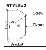
**STYLE #2** - Insert one screw into the mounting bracket - do not tighten yet. Tuck electrical wires into outlet box and position fixture over the mounting bracket. Line up the screw in the bracket to the "7" hole on the fixture. Slide fixture to secure in place. Insert remaining screw. Tighten both screws to secure.
